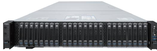
The NF8260M5 is a 2U 4socket rackmount server designed by Inspur based on the latest Intel® Xeon® scalable processor series. It has reached the industry-leading computing density by supporting up to 4 Intel® Xeon® scalable processors as well as 48 \* DDR4 DIMMs and 24\*2.5" hard drives in a 2U space.
